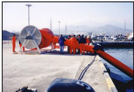
AirBoom has very compact storage dimensions, especially when stored on powered boom reels.
