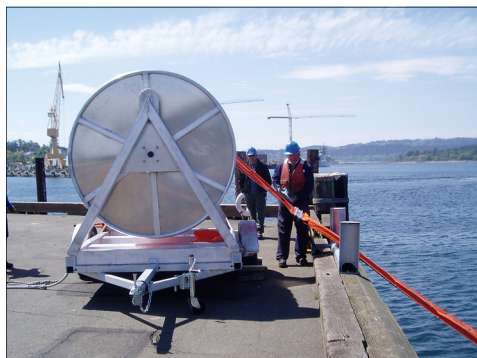
BoomReels may be trailer-mounted for ease of transportation from storage location to spill site
