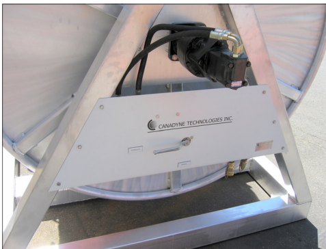
BoomReel 7296 showing direct-drive hydraulic drive motor and emergency bypass control.
